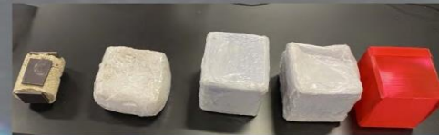
Images 5. The brick with cube container and layers of PETG could withstand a force approximately 7,100 Newtons without being compressed.
