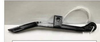
Long Arm V.1 made of nylon carbon. This arm snapped after 8 kg.
