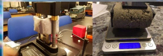
Image 6 and 7. The sucrose gelatin concrete could withstand a force approximately 7,100 Newtons without being compressed.
